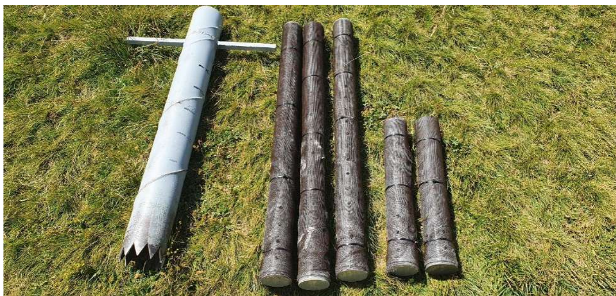
Figure 15 Piezometers and driller for their positioning in the soil ©Marija Chobanova
