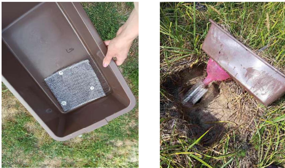
Figure 24 Design of the lysimeters ©Dragana Pelikudovska Trajchevska
